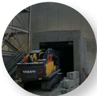
The remote control capacities of the machine allow full wireless operation of the units ISO controls and also are able to run auxiliary electric over hydraulic circuits. It is fitted with (3) CC TV conventional cameras for the operator to remotely view as well as (1) infrared camera for low visibility environments.
